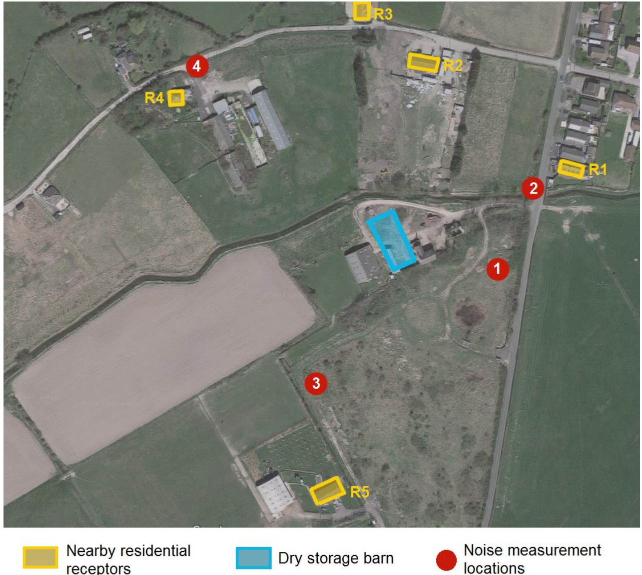
Figure 2: Site plan showing dry storage barn, nearby receptors and noise measurement locations (NMLs)
